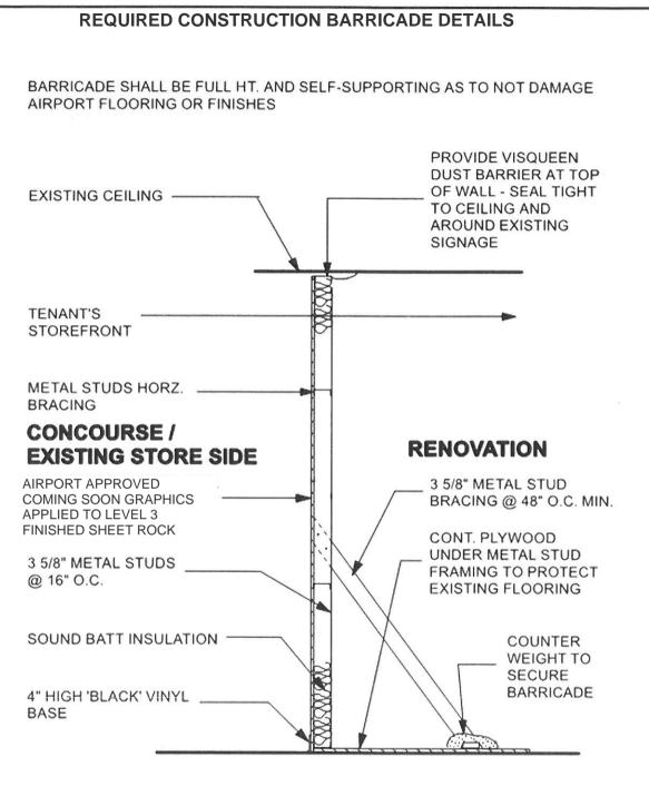
1 DETAIL TEMPORARY CONSTRUCTION BARRICADE
